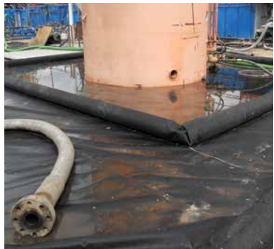
Passive containment — like this drilling site berm — doesn't have to be permanent, just effective.
