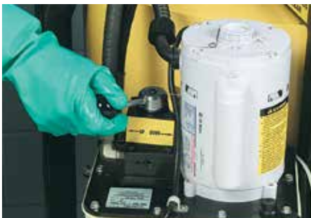
4. Move directional lever on electric pump to the down position and depress operation button to compact. Continue to compact until the pump stops (reaching maximum pressure).
