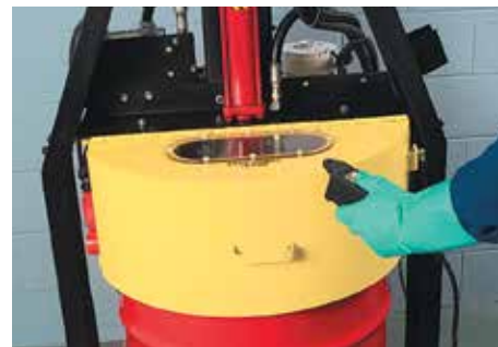
5. To raise the ram, release button to stop, move directional lever on air hydraulic pump to the up position and depress operation button.
