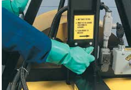
2. Tilt unit back with drum in place to facilitate loading.
