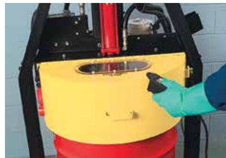
5. To raise the ram, release button to stop, move directional lever on electric pump to the up position and depress operation button.
