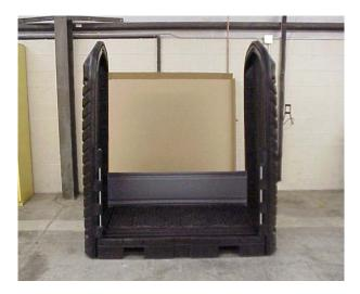
Step 5Take another rod assembly and insert it through the front bottom<br/>hole in the left sidewall. Slide the black pipe(14) over the rod<br/>assembly. Then push the rod through the right sidewall and place a<br/>washer(10) and a nylon nut(12) on the rod assembly. Tighten nut ½"<br/>onto threaded rod.
