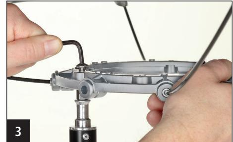
**Step 3:** Turn entire assembly upright and fasten to tripod stand using included 5/32" Allen wrench, bolt and washer. Avoid overtightening. Only two holes will accept bolt; either can be used.
