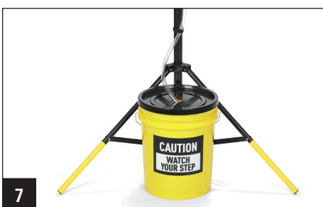
**Step 7:** Place diverter directly below leak and position bucket so caution message is visible. Attach lid to bucket and insert hose into hole. Monitor collected water and empty as needed.
