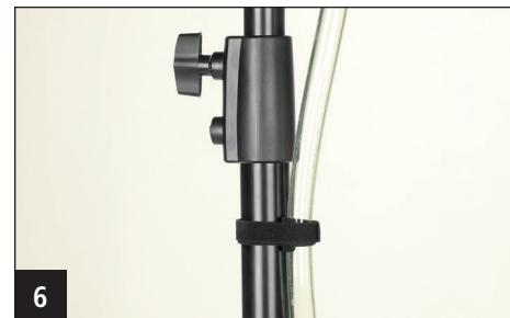
**Step 6:** Secure hose to tripod using provided hose ties. Continue to adjust height of diverter as you add ties.
