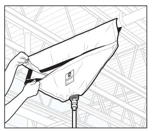
Reattach matching hook and loop closures in each corner, then reattach all other closures until unit fits snug to pipe.
