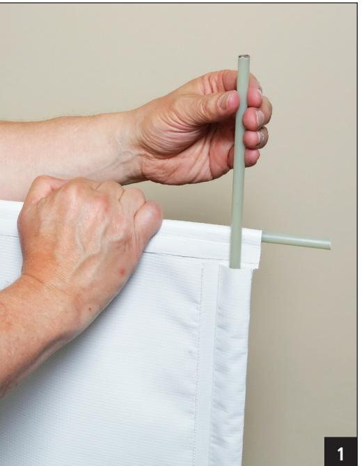
With drain elbow facing up, insert the two longer rods (54") into the pockets running parallel to drain elbow. Flip tarp over and insert the shorter rods (49") into remaining pockets.
