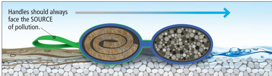
**Proper Installation** – To increase efficiency and product lifespan, the green handles should always face the source of pollution.
