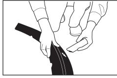
3. Insert gray notched pipe into port, with opening facing the floor.
