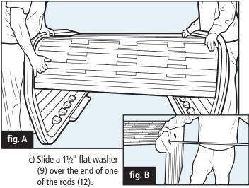
**NOTE:** All thread rods (12) will have an acorn nut (10) installed at the factory with thread lock applied.
