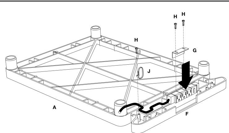
Attach electric outlet **F** to top shelf **A**, secure with L bracket **G** and cable lock **J**. Loop outlet cable **F** through cable lock **J** and the inserts on shelf **A**. Screw L bracket **G** and cable lock **J** onto top shelf **A** with screw **H** and a philips screwdriver.
