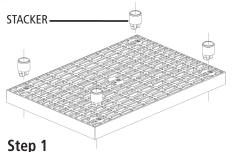
Set completed base unit upright and insert stackers in sockets as shown.
