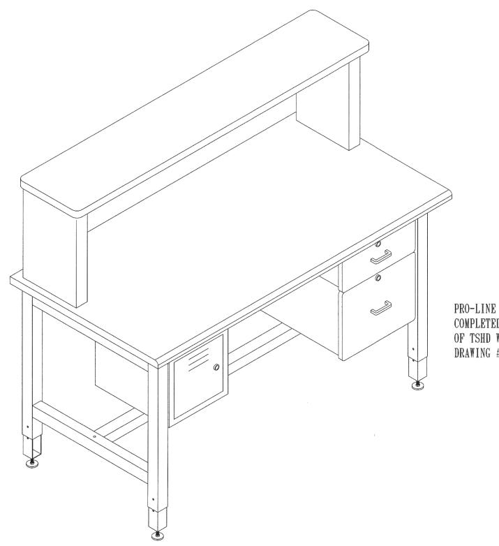
PRO-LINE COMPLETED DRAWING OF TSHD WITH PLASTIC LAM. DRAWING #A7715
