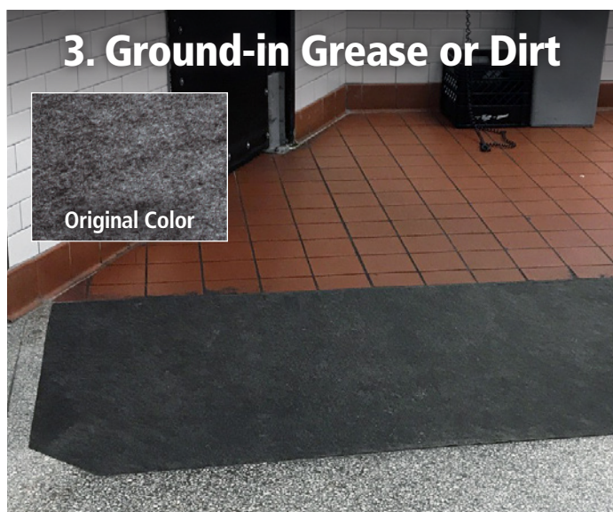
Mats that darken and/or change color from grease and dirt have reached the end of their lifespan: REPLACE.
