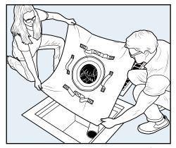
2. Place Drain Filter over opening. Filter fabric should overlap drain at least 3" on all sides.
