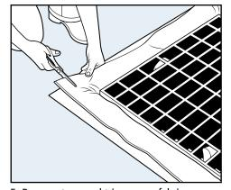
Remove tape and trim excess fabric, keeping roughly 3" of material on all sides.
