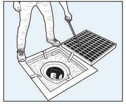
6. Replace drain grate overtop installed PIG Storm Drain Filter.
