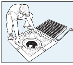
4. Place the PIG Storm Drain Filter directly on grate lip inside of storm drain.
