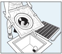
3. Expand or collapse the PIG Storm Drain Filter frame to fit intended storm drain size.
