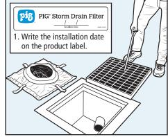
2. Remove drain grate and clean any existing sediment off grate lip inside of storm drain.
