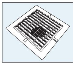
7. For best visibility and to keep filter securely in place, ensure green straps are not caught beneath storm drain grate.
