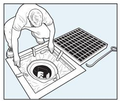
5. Pull frame flush against walls of storm drain to ensure a tight seal.
