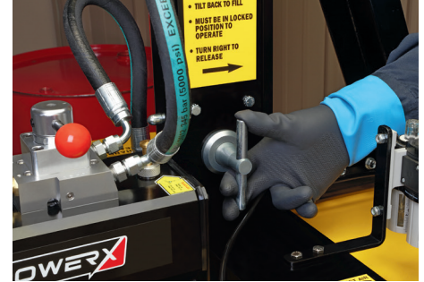
3. Return to upright locked position and close safety cover.
