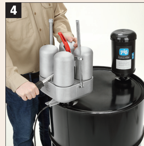
4. Raise ratchet clamp until it contacts cover, pull lever to tighten. Do not overtighten ratchet clamp (three clicks only). Press handle to raise pins and puncture cans. Lift handle after puncturing. Allow cans to fully drain. Remove cans and position cover back into fully closed position.
