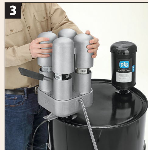
3. Unlock cam-lever clamp to lower cover and close puncturing unit.
