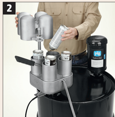
2. Insert one domed can into each chamber of puncturing unit. All cans must be the same height.
