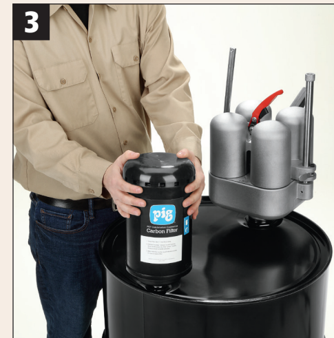
3. Thread combination filter into 3/4" bung. Press "power" button on Timestrip Indicator to start tracking 3-month service life.
