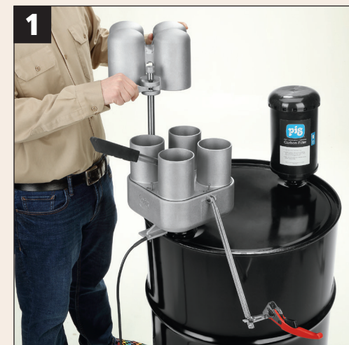
1. Disengage and lower ratchet clamp on right side of puncturing unit. Unlock cam-lever clamp on left side of puncturing unit to slide cover up to the open position. Lock cam-lever clamp to hold lid in place.
