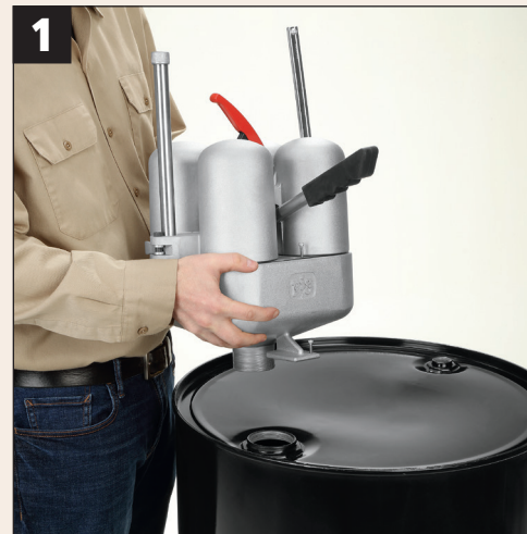
1. Thread 4-can puncturing unit into 2" bung until support plate touches rim of drum.
