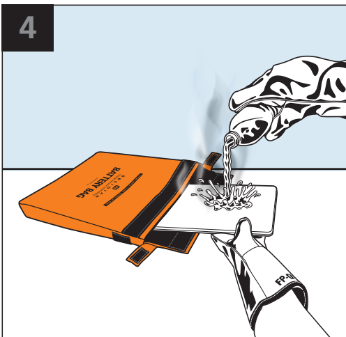
4 Water is not required, but if your safety protocols call for cooling the threat with water, do so before sealing the threat inside the orange bag.
