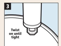
**3.** Thread Combination filter into <sup>3</sup>/<sub>4</sub>" bung. Activate Timestrip<sup>™</sup> Indicator by pressing "power" button to start tracking 3 month service life.
