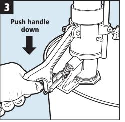
**3.** Depress handle to puncture the can and relieve the pressure. DO NOT release until all of the contents are dispersed.
