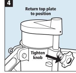
**4.** Remove can and position top plate back into position and tighten knob to seal drum (reinsert sleeve if removed).
