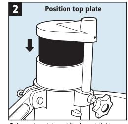
2. Lower top plate and firmly seat, tighten lock knob.
