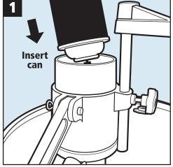
1. Insert domed can (jumbo/standard/mini), lower top cover to hold can firmly in place, tighten knob. Use sleeve for standard cans, remove for jumbo cans.
