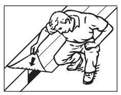
3. Place product over the drain, tacky side down, making sure it overlaps all sides of the drain by at least 3 inches.
