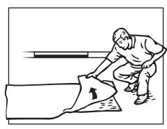
Remove the clear protective film from the product and set aside for reuse.
