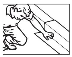
4. Press firmly along the edges and drain face to secure the seal.
