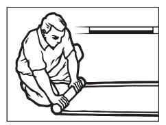
6. When the product is completely dry, replace the protective film and return to box the same way it was packaged. Store away from direct sunlight.
